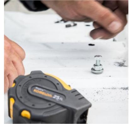
Assemble (1) Jack-Nut, 1/4" Flat Washer, 5/16" Nut & 1/4"-20 Bolt. Insert jack-nut assembly into holes of tailgate. Using a 1/2" wrench on nut & 7/16" wrench on bolt head, hold 1/2" wrench & tighten bolt until tight - this will cause the jack-nut body to collapse to form legs which grip the inside of the mounting surface; leaving a permanent, reusable threaded insert. Un-screw flat washer, nut & bolt and repeat process for the remaining (5) holes.
