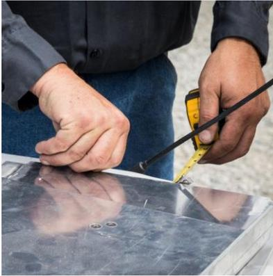
Place the base plate onto the tailgate with the flanges down & the key slot running vertically. The plate should be approximately 1" from the front edge of the tailgate and 1 1/2" from the side edge of the tailgate.
