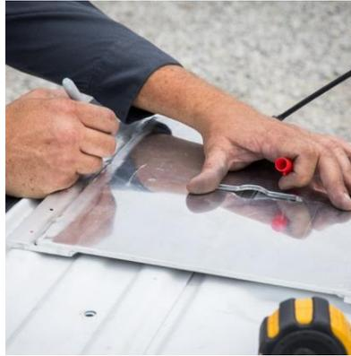
Locate & mark (6) hole locations on the Tailgate and on the Base Plate where the bolts will be located; (4) of the (6) locations are recommended to be in the ribs of the tailgate. Using a 7/16" drill bit, drill (6) holes in the Tailgate. Move the Base Plate to a safe drilling location, free from obstruction, and pre-drill the (6) holes with 1/4" drill bit.
