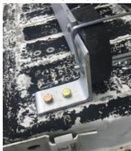
To use the ladder, rotate the ladder 90 degrees off the tailgate, aligning straight with the base plate. Slide the ladder completely out to the fully extended position & lower to the ground. Assure ladder is fully extended and snug to the ground. Raise handle & allow it to drop securely into the holding slot.
