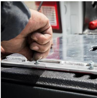
Align pre-drilled Base Plate holes over newly installed jack-nuts in tailgate. Insert a 1/4" Lock Washer and 1/4"-20 Bolt using 7/16" wrench until tight into (6) jack-nuts.
