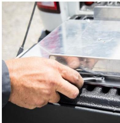
Align scribed arrow on top of Base Plate with scribed arrow on Swivel Plate to allow key on underside of Swivel Plate to drop into key slot of Base Plate. Rotate Swivel Plate placing slots over edge of tailgate to install ladder.
